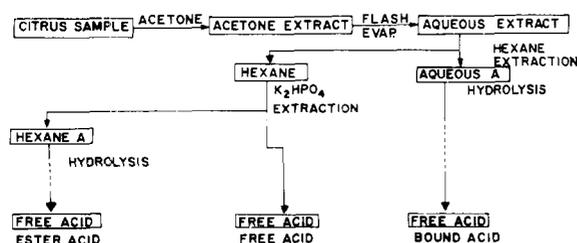
Figure 2. Schematic diagram indicating separation of residue fractions
