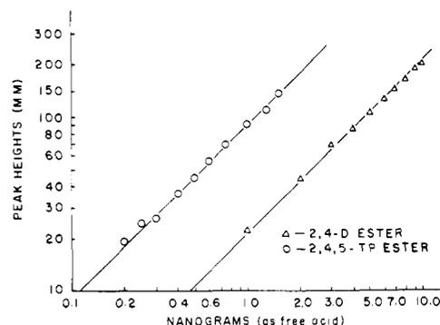
Figure 3. Standard curves for butoxyethyl esters of 2,4-D and 2,4,5-TP
